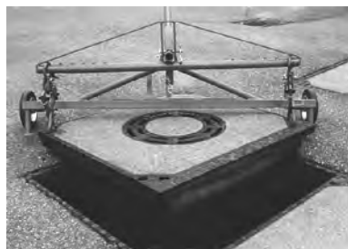
Manhole covers lift truck HK for cable shaft covers, rectangular and square manhole covers as well as all current round covers up to max. Ø 115 cm.
